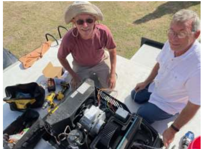
Roger and Tim installing a SoftstartRV in the AC unit on Jan’s 2021 Grand Design Imagine
